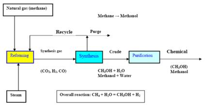
Figure 2. Schematic diagram shows methanol production (Omer, 2006).
