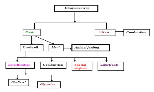
Figure 9. Flow chart of biodiesel production (Omer, 2006).
