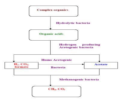
Figure 3. Biogas production process (Omer, 2003).
