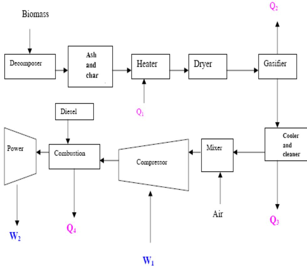
Figure 7. Advanced biomass power with diesel engine (Omer, 2006).
