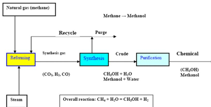
**Figure 2.** Schematic diagram shows methanol production (Omer, 2006).
