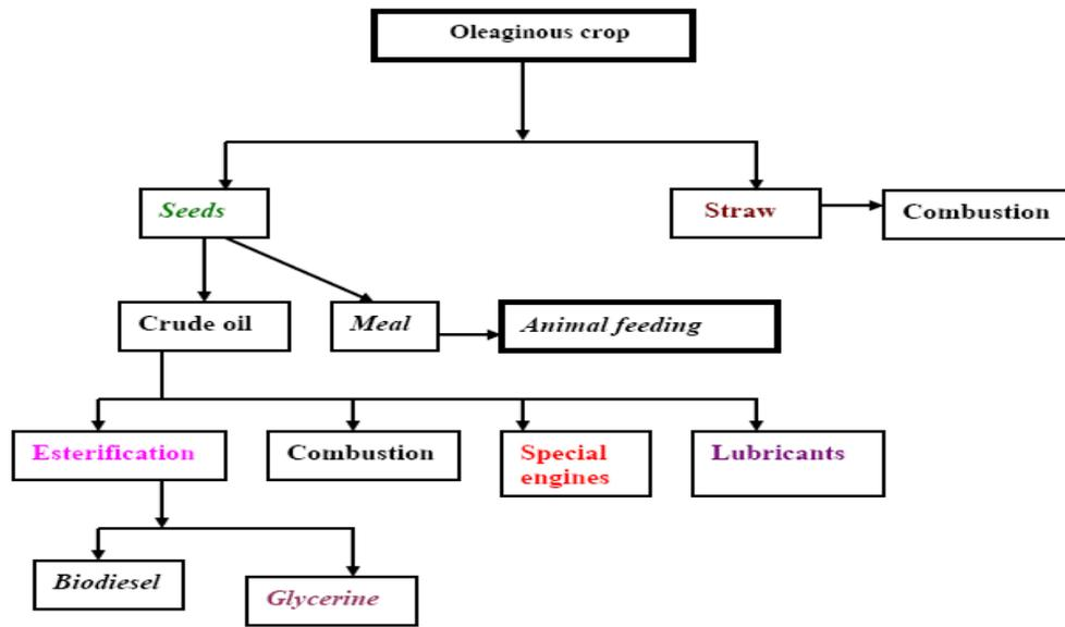
Figure 9. Flow chart of biodiesel production (Omer, 2006).
